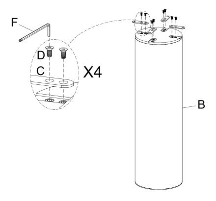
2 Attach the Column Base (B) to the Top Panel (A) using Bolt (E) through the Metal Bracket (C) with the Allen Key (F).
